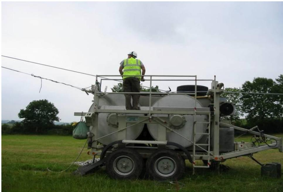
Figure 7.1: Puller – Tensioner machine
